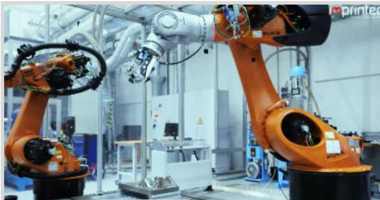
In this project, Fraunhofer IPA and Imprintec integrated the i3D technology into a 6-axis industrial robots. Successful tests were conducted on both individual and serially manufactured components.
